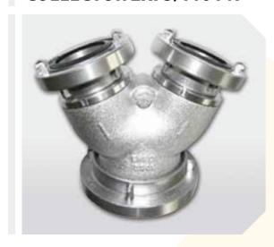
Collector allows delivery of water to the 110 hose from the two power sources of the 75 hose. The backflow valve allows for automatic shut-off of one the inlets in the case of a large differential power pressure.
